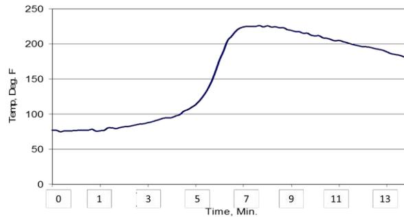
The figure below shows the exothermic curve at 23°C with a volume ratio of 10:1 and a weight of 10gr.
